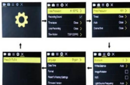
Press the OK Button to enter the settings menu. Repeatedly press the Power/Mode Button to cycle through options and press the OK Button to select desired option.
